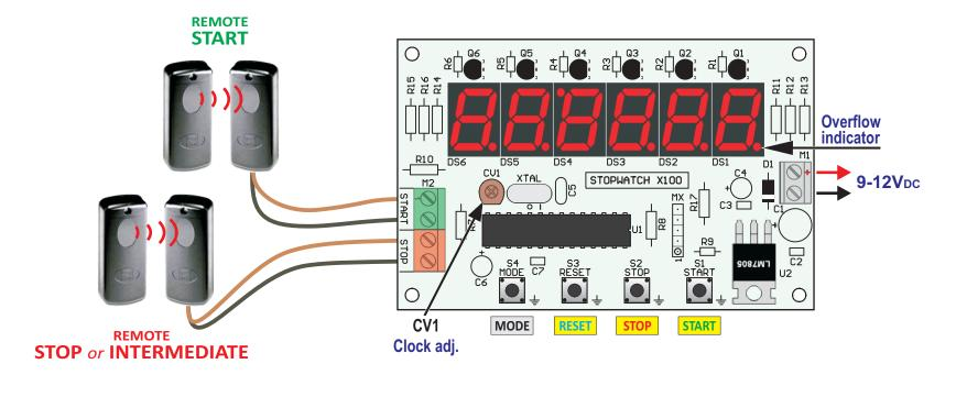
SENSORs or PHOTOCELLs Contacts must be Normally Open (N.O.)
